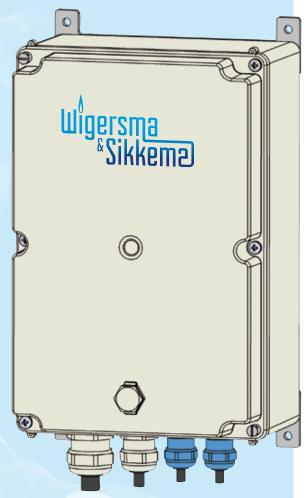
UNILOG 300 is a GSM /GPRS modem for UNIGAS with in addition an optional standalone data logger function. Signal inputs are equipped with an EX-barrier. This allows UNILOG 300 to be connected directly with devices like UNIGAS or a gas meter in a hazardous area. An internal antenna is standard equipment, connection with an (optional) external antenna is possible. UNILOG 300 is available in a battery powered version and a mains operated version.
