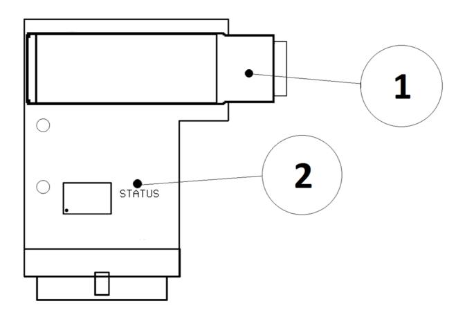
Figure 2. Connector and LED on the PSTN module
