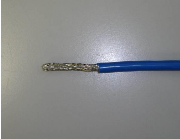
1: Remove the sheath over 35 mm
